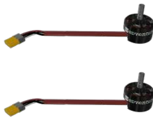
CCW Motors Counterclockwise (Red Wire)
