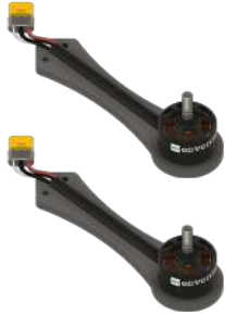
CW Motors Clockwise (Black Wire)
